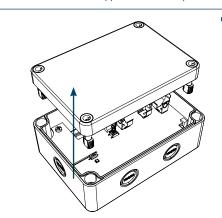
Remove the lid from the back box, removing the screws on the corners.
