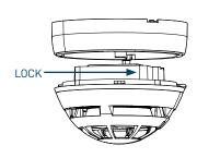
• Ensure you replace the battery cover as this forms part of the detectors anti tamper protection and refit the detector locating it into the base twisting clockwise.
