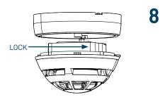
• Ensure you replace the battery cover as this forms part of the detectors anti tamper protection and refit the detector locating it into the base twisting clockwise.
