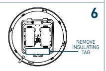
Remove the batteries' insulating tab ensuring the batteries are kept in their lodgement.
