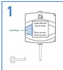
To open the MCP, rotate the lock door counterclockwise and use the supplied key
