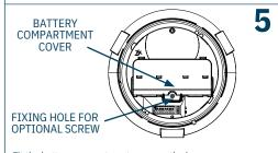
Fit the battery compartment cover on the base.
